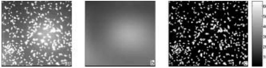
Fig. 2. Original image before background correction (a), the fitted spline surface of the background (b) and the image after background subtraction (c). Note that the intensity scale (same for all images) has been set to enhance the contrast of the darker parts of the images.
