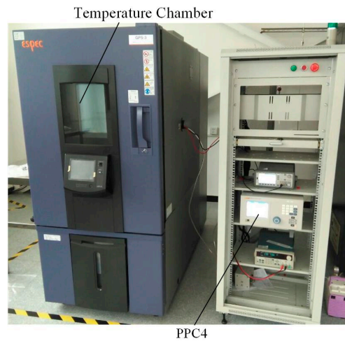
Figure 12. The calibration system for the sensor.
