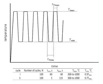
**Figure 7.** Schematic representation of the two thermal cycles to which the  $TiAl_{1-x}Cr_xN$  + tool steel was subjected to determine the minimum working temperature by which surface oxidation started to form on the coating.
