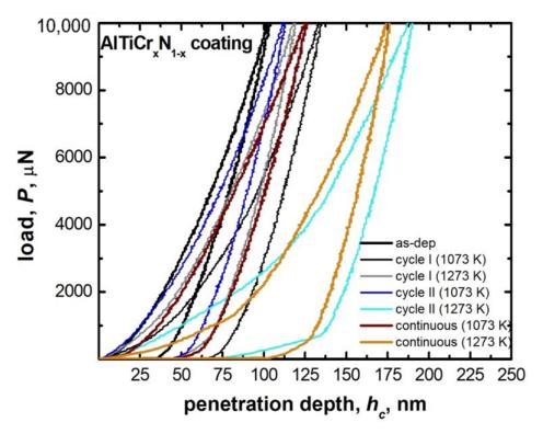
**Figure 9.** Nanoindentation load-displacement curves of AlTiCr<sub>x</sub>N<sub>1-x</sub> coating after cycles I, II (see Figure 6), and continuous exposition to 800 and  $1000 \,^{\circ}$ C.
