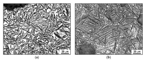
**Figure 12.** Typical microstructure of ADI (austempered ductile iron) materials: (a) plate-like ausferrite morphology  $(400 \, ^{\circ}\text{C}/2 \, \text{h})$ ; (b) acicular morphology  $(300 \, ^{\circ}\text{C}/2 \, \text{h})$ .
