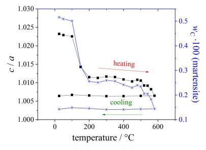
**Figure 4.** Tetragonality c/a of martensite (black curve with squares) and carbon mass fraction in martensite (blue curve with squares) versus temperature during a heating/cooling cycle.
