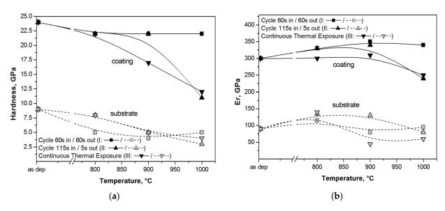
**Figure 10.** Hardness, H, (a) and  $E_r$  (b) of AlTiCr<sub>x</sub>N<sub>1-x</sub> coating after thermal cycles I, II (see Figure 2), and continuous exposition for 24 h to the upper temperature range (1000  $^{\circ}$ C). The corresponding behavior of the substrate tool steel is also reported for comparison.
