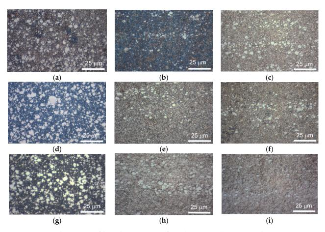
**Figure 6.** OM (optical microscopy) of the  $TiAl_{1-x}Cr_xN$  coating after cycle I ( $\mathbf{a}$ , $\mathbf{d}$ , $\mathbf{g}$ ); cycle II, ( $\mathbf{b}$ , $\mathbf{e}$ , $\mathbf{h}$ ); and continuous exposition (24 h) ( $\mathbf{c}$ , $\mathbf{f}$ , $\mathbf{i}$ ) at maximum testing temperature of 800 °C ( $\mathbf{a}$ – $\mathbf{c}$ ); 1173 K, ( $\mathbf{d}$ – $\mathbf{f}$ ); and 1000 °C, ( $\mathbf{g}$ – $\mathbf{i}$ ).
