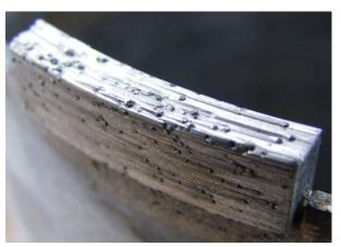
**Figure 15.** Examples of sections of the newly made saws. Diamond segments: the segment dimension is dependent on the saw diameter. For the presented  $\emptyset$ 450 mm saw, the segments dimension is  $40 \times 4.2 \times 10$  mm.
