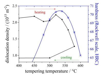
**Figure 5.** In situ dislocation density in martensite derived from the microstrain (black curve with triangles) versus temperature during a heating/cooling cycle and ex situ Rockwell hardness in martensite (blue curve with stars).
