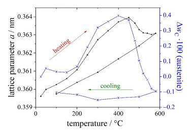
**Figure 3.** Lattice parameter a of austenite (black curve with small triangles) and change in carbon mass fraction  $\Delta w_C$  (blue curve with stars) versus temperature during a heating/cooling cycle.
