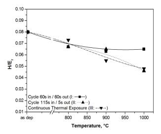
Figure 11. H/Er vs. temperature for cycles I, II, and continuous exposure.
