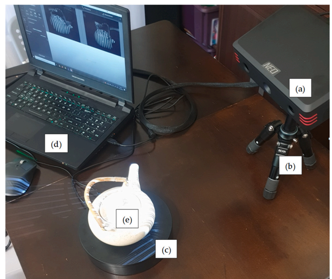
Fig. 1. 3D digitization of an object with a RangeVision NEO scanner: (a) Scanner; (b) Tripod; (c) Rotating table; (d) Laptop with software; (e) Scanned object.
