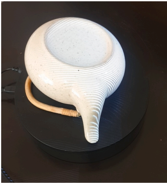
Fig. 2. Scanned object illuminated by structured light.
