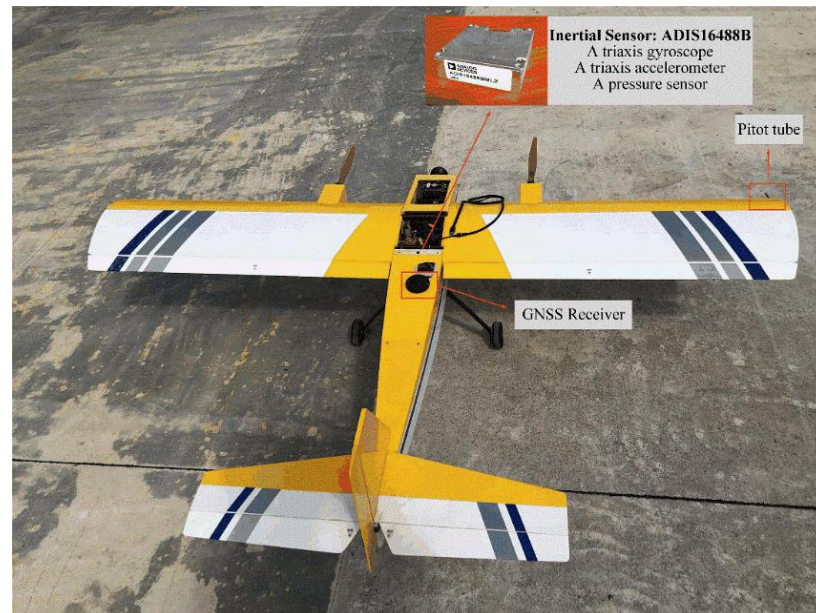
Figure 4. The experimental platform of the small fixed-wing UAV.
