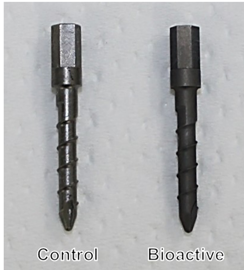
Fig 1. Pedicle screws (2.5 mm in diameter, 14 mm in length) were prepared from Ti-6V-4Al alloys and bioactivated by NaOH-CaCl 2 -heat-water treatments. Control: untreated pedicle screw. Bioactive: bioactive pedicle screw.
