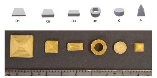
**Figure 1.** Designed geometries (from left to right): cube 1 (Q1), cube 2 (Q2), cube 3 (Q3), hollow cylinder (HC), cylinder (C) and pyramid (P). Upper image: CAD-Design, lower image: printed geometries of SA/V ratio  $1.5 \text{ mm}^{-1}$ .
