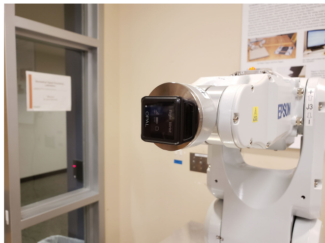
FIGURE 4. Epson C3 robotic arm used for algorithm verification. The inertial sensor is attached to the end effector using a custom 3D-printed jig.
