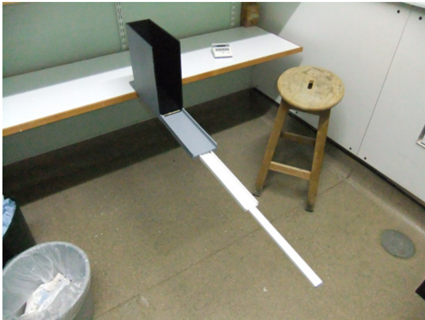
Figure 1. The mouse successive alleys apparatus. It is made of painted wood and is clamped on to the bench.
