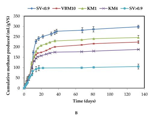
**Figure 4.** Cumulative methane production for different dry fractionation process of T olive pomace from three-phase extraction process: (**A**) Milling pretreatments and (**B**) dry separation process (electrostatic and sieving).
