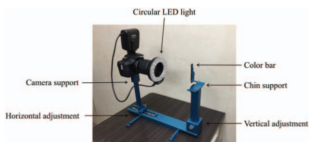
Figure 2. Components of the automatic tongue diagnosis system.
