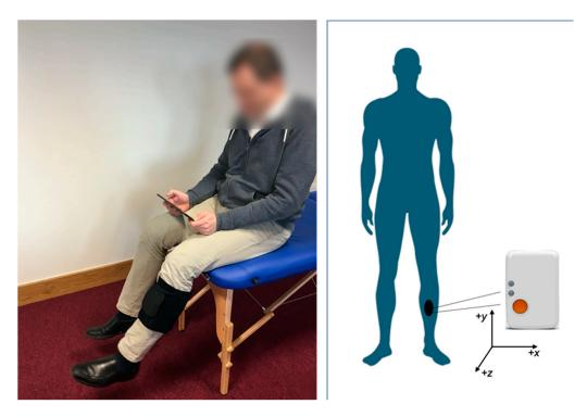
**Figure 1.** User setup and IMU orientation of the biofeedback system consisting of a single IMU and associated Android tablet application (figure adapted from [23]).
