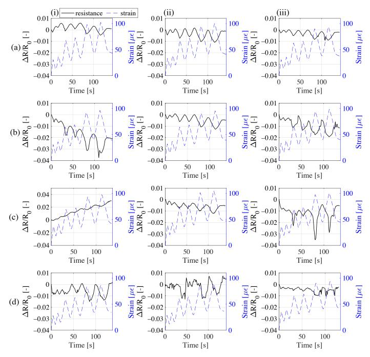
**Figure 9.** Relative change of resistance versus strain time histories each of the three samples belonging to the set of; (**a**) 1-32CMF0G; (**b**) 1-32CMF10G; (**c**) 1-32CMF20G; (**d**) 1-32CMF30G.
