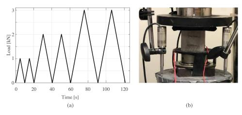
**Figure 8.** (a) The load time history, F(t); (b) the setup of the electromechanical tests.
