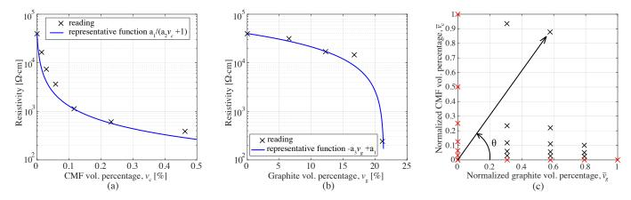
**Figure 6.** (a) Function  $f_c$  versus CMF-only experimental data; (b) function  $f_g$  versus CMF-only experimental data; and (c) polar coordinate system.
