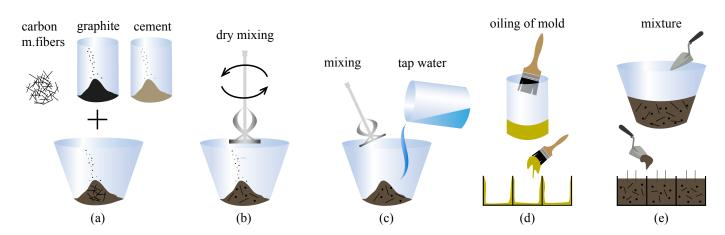
**Figure 2.** Preparation steps for cubic samples with G+CMF hybrid inclusions; (**a**) combination of CMF, G, and cement; (**b**) dry mechanical mixing of materials; (**c**) addition of water and mixing until homogeneity; (**d**) preparation and oiling of metal molds; and (**e**) the pouring of compound into molds and placement of steel electrodes.
