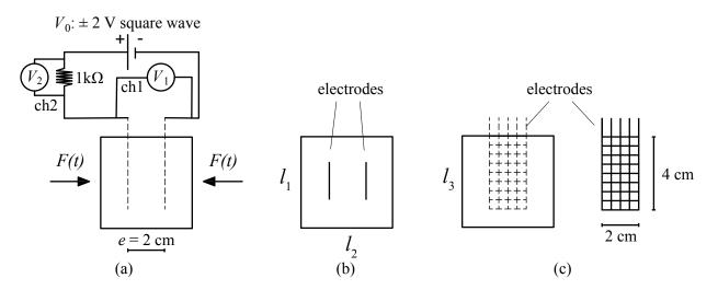
**Figure 4.** The sample and electromechanical setup illustration; (**a**) general view of the cube samples together with electrodes, electric circuit with channels and voltage readings, and, the applied load F(t); (**b**) the top view of the sample and the mutual distance of electrodes; (**c**) side view of sample and electrodes.
