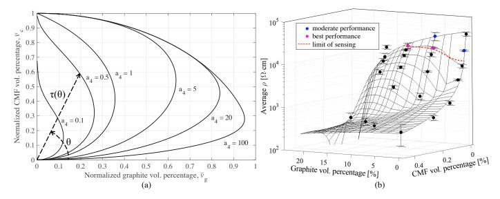
**Figure 7.** Illustrations regarding to optimization of resistivity surface; (a) The distributions of interpolation metric,  $\tau$ , with respect to changing  $a_4$ ; (b) the obtained resistivity surface together with performance evaluation and observed limit of sensing.
