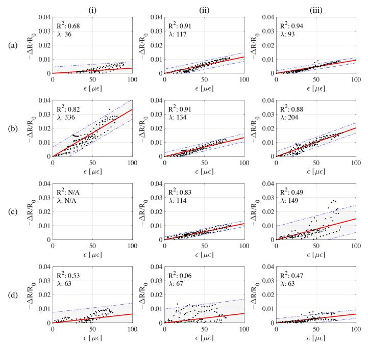
**Figure 10.** Discrete data points of fractional change of resistance vs. change of strain time histories with the best fitted line for all the samples; (a) 1-32CMF0G; (b) 1-32CMF10G; (c) 1-32CMF20G; (d) 1-32CMF30G.
