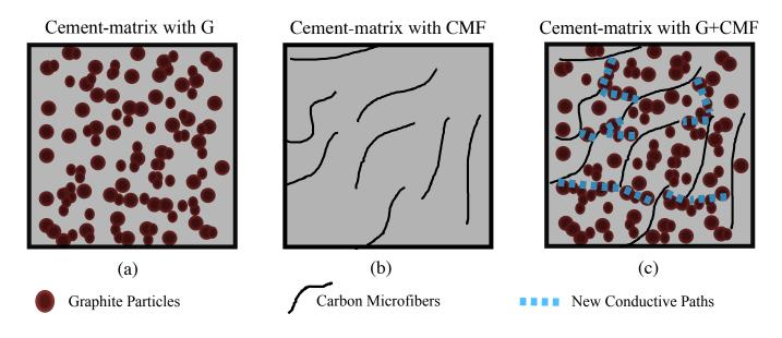
**Figure 1.** Illustration of accelerated percolation using hybrid filler: (**a**) G only; (**b**) CMF only; and (**c**) hybrid G+CMF filler showing a formed conductive path.
