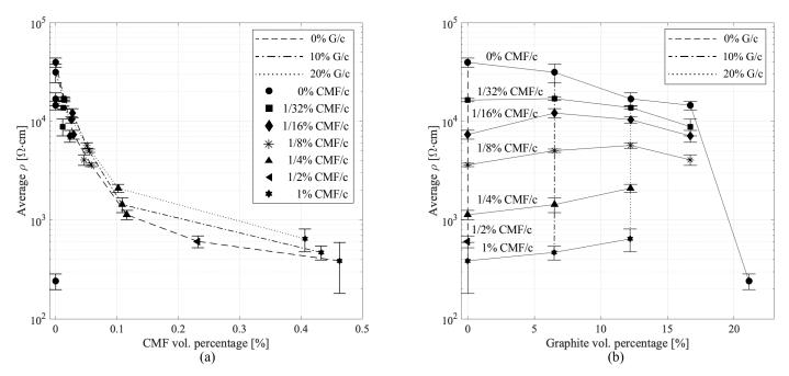
**Figure 5.** Sample resistivity  $\rho$  as a function of doping level showing average values, and the maximum/minimum values denoted by the bar. (a) 3D view plotting the evolution of  $\rho$  per constant G/c; and (b) evolution of  $\rho$  per constant CMF/c.
