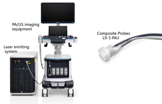
Fig E2. Photoacoustic/ultrasound imaging system and imaging probe (L9-3PAU, center frequency 5.5 MHz).
