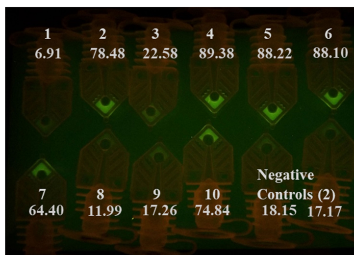
Figure 2. PCR tubes after a RT-PCR run using 3 \mu L of untreated transport media samples. Seven out of ten samples can be identified as positive COVID-19 patient samples by comparing results with negative controls. The RT-PCR run was completed in 12 min, and the RT-PCR protocol was (90 s/30 s/40 × (6 s/9 s)). The signal intensity measured by ImageJ is listed under the sample number.
