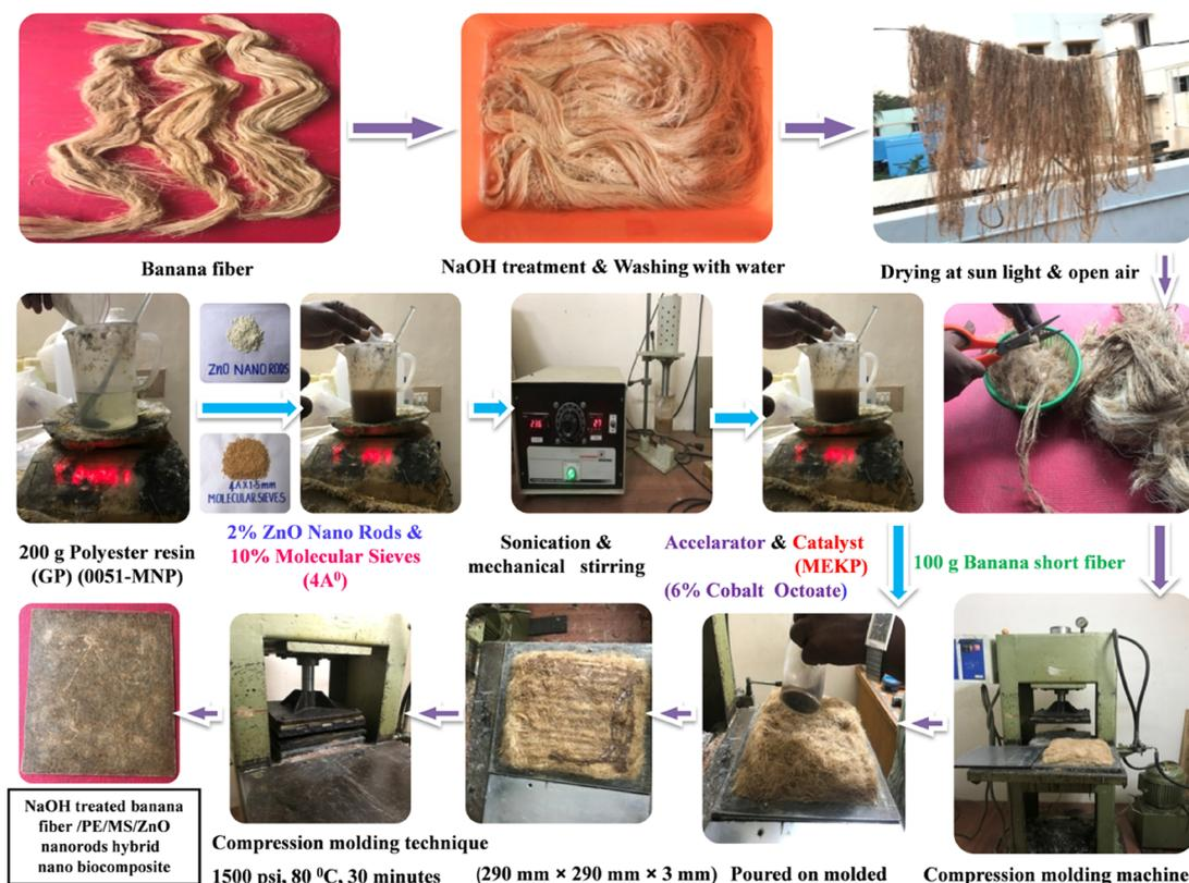
**Figure 9.** Preparation of NaOH-treated randomly oriented short BF/PE/MS/ZnO hybrid nanobiocomposite by the compression molding technique.
