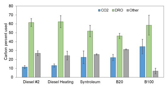
**Figure 1.** Percent carbon mass balance for different fuel types at the end of the experiment based on respiration (CO<sub>2</sub>) and Diesel Ranges Organics (DRO) measurements by GC-MS. Conditions: 20  $^{\circ}$ C; 300 mg N, 1 kg of sand; 2000 mg of diesel, heating diesel, Syntroleum, B20, and pure fish biodiesel (B100). Values represent means  $\pm$  SE.
