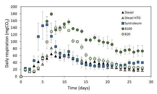
**Figure 2.** Daily respiration (CO<sub>2</sub>) values for conventional diesel, heating diesel (HTG), Syntroleum, B20, and B100. Conditions:  $20\,^{\circ}$ C;  $300\,\text{mg}$  N, 1 kg sand;  $2000\,\text{mg}$  of selected fuel. Values represent means  $\pm$  SE.
