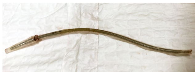
FIGURE 2 Intraprocedure photo from the cardiac resynchronization therapy device implant in 2018 showing the proximal explanted fragment of the fractured epicardial lead
