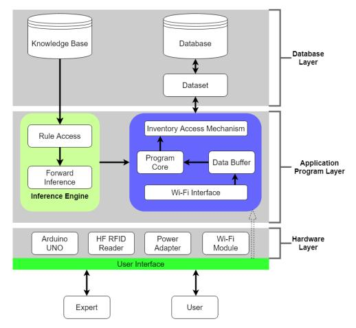
Figure 2. The three-layer framework of the material inventory management system.
