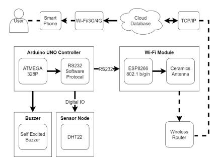
Figure 6. The hardware framework of the sensing node.
