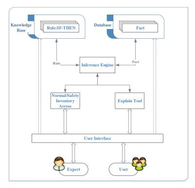
Figure 3. The components and operation processes of the expert system.
