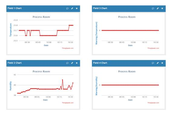
Figure 9. Temperature and humidity curves and alarm curves recorded on the ThingSpeak website.
