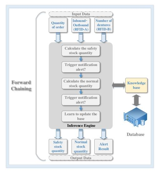
Figure 4. The architecture of the expert system.
