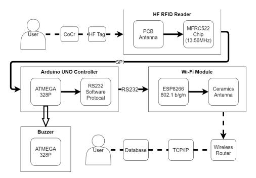
Figure 5. The hardware framework of material inventory management.
