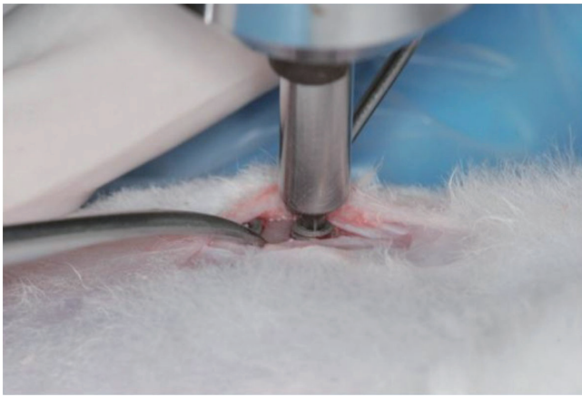
Fig. 2. An MGT-12 digital torque gauge (Mark-10 Corp, New York, NY, USA) was used to measure the removal torque with a connector specifically made to connect the torque gauge and the fixture.
