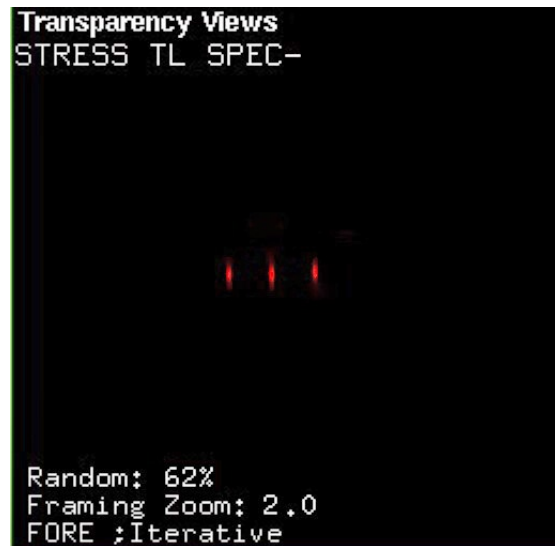
FIG. 2. The SPECT image of three YAS glass seeds that were placed into the cylindrical water phantom.
