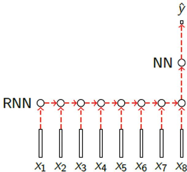
**Fig. 6** An unrolled view of RNN across the time-step dimension. Here, RNN can be a layer of Simple RNN or LSTM. NN is a layer of densely connected NN with softmax activation.  $X_n$  are the inputs across  $n$  timesteps.  $\hat{y}$  is the output. LSTM, long short-term memory; NN, neural networks; RNN, recurrent neural network.
