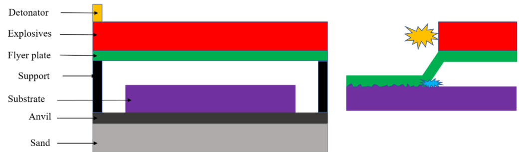
Figure 15. Schematic of the EW technique.
