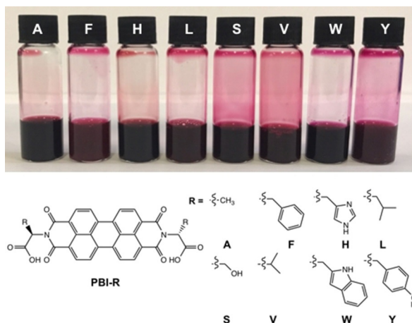
Figure 1. (Top) Photograph of PBIs in solution. (Bottom) Structures of the PBIs; the letter represents the amino acid used for functionalisation.
