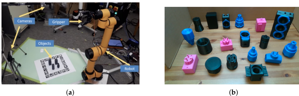
Figure 2. (a) Our experimental setup. The images from the top view camera provide an initial estimate of the ROI and the images from the perspective view camera provide the final object detection and recognition. (b) Some of the textureless objects we used. All of the objects are 3d printed from [25].
