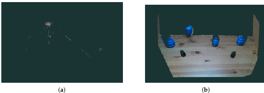
Figure 5. (a) Original point cloud captured by a RGB-D sensor, (b) the same point cloud after removing the unwanted region.
