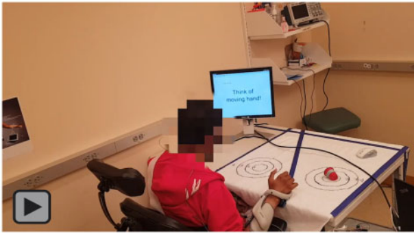
Video 3 Functional task to transfer light object. The subject successfully used the BCI to trigger FES allowing the subject to grasp and transfer a cup between targets placed in front of the subject.
