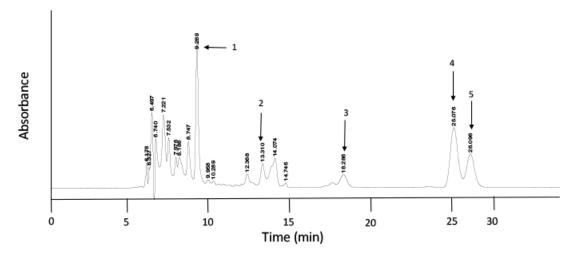
**Figure 2.** HPLC elution profile recorded at 460 nm showing the separation of the  $\beta$ -carotene and the geometric isomers of lycopene from an extract of plasma taken from a non-smoker:  $\beta$ -carotene (1); (13Z)-lycopene (2); (9Z)-lycopene (3); (all-E)-lycopene (4); and (5Z)-lycopene (5). The details for the extraction and separation are described in the methods section.
