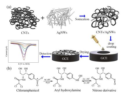
**Figure 1.** (a) Schematic diagram of electrochemical detection of CAP based on CNTs/AgNWs nanocomposites. (b) The proposed reaction scheme of redox reaction of CAP during electrochemical detection.
