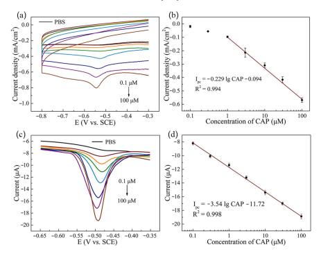
**Figure 5.** (a) CV curves of CNTs/AgNWs electrodes with various concentrations of CAP and (b) the peak current density as a function of CAP concentration (background subtracted). (c) DPV curves of CNTs/AgNWs electrodes for CAP detection and (d) the corresponding peak current versus CAP concentration.
