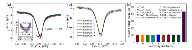
**Figure 6.** (a) DPV curves of CNTs/AgNWs electrodes for 100  $\mu$ M CAP detection; the inset graphic depicts an enlarged view in the potential range between -0.53--0.47 V. (b) The reproducibility of CNTs/AgNWs electrodes. (c) Good selectivity of our electrodes against interferences.
