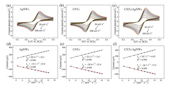
**Figure 4.** (**a**–**c**) CV of AgNWs, CNTs, and CNTs/AgNWs electrodes in 10 mM  $[Fe(CN)_6]^{3-/4-}$  and 0.1 M KCl electrolyte solution at scan rates (*v*) from 20 to 200 mV s<sup>-1</sup>. (**d**–**f**) Linear plots of  $I_{pa}/I_{pc}$  vs. *v*.
