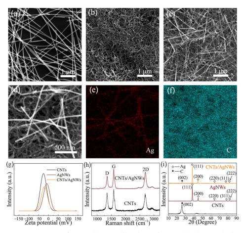
**Figure 2.** SEM images of AgNWs (**a**), CNTs, (**b**) and CNTs/AgNWs (**c**). (**d**) Regional enlarged view of the nano-intertwining structure of (**c**). The EDS mapping of element distribution of Ag (**e**) and C (**f**). (**g**) Zeta potential of CNTs, AgNWs, and CNTs/AgNWs dispersion. Raman spectra (**h**) and XRD patterns (**i**) of CNTs/AgNWs nanocomposite.
