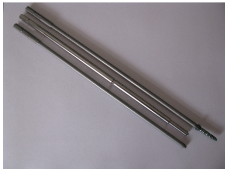
FIGURE 3: Image of the three reverse threaded screw drivers used. The top driver was successful in removing the screw but cold-welded to the interface. The bottom two drivers broke distally when used unsuccessfully on the remaining screws.
