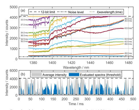
**Figure 2.** Examples of detected spectrometer signals (1 vol. % 1-MN in isooctane, 1 MPa 900 K,  $\tau_{\rm res} = 315$  ms,  $X_{\rm H2O} = 0.98$ %). (a) Typical transmission spectra *I* (colors represent single frames at manual selected time steps, smoothed) with temporal variations in signal intensity; and, (b) temporal course of spectral averaged signal intensity and fraction of evaluated (threshold filtered) spectra.
