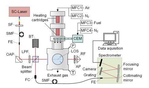
**Figure 1.** HTC<sup>2</sup> calibration flow cell and the optical supercontinuum laser absorption spectroscopy (SCLAS) configuration. Optical components: spectral filter (SF), single mode fiber (SMF), fiber end (FE), off-axis parabolic mirror (OAP), longpass filter (LPF), beam trap (BT), aperture (AP), retroreflector (RF), and fiber collimator (FC).
