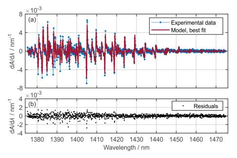
**Figure 3.** Example for spectra evaluation using NLLSQ curve fitting. (**a**) Best fit for an example dataset (1 vol. % 1-MN mixture consumption resulting in  $X_{H2O} = 0.25\%$  at p = 1.5 MPa, T = 850 K); (**b**) residuals.
