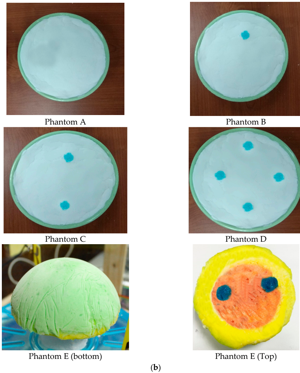
Figure 12. The architecture and a different component of the proposed experimental breast imaging system; (a) block diagram (b) breast phantoms.
