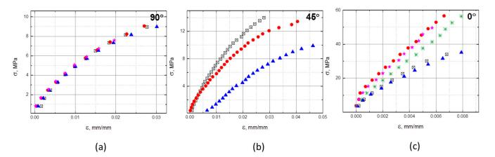
**Figure 4.** Results of tensile tests on the double layer reinforced composite in three directions: (**a**) in the 90°, (**b**) in the 45° direction and (**c**) in the 0° direction, with respect to UD fibers orientation (a data set for each tested specimen is presented with a different symbol).
