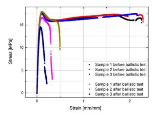
Figure 8. Tensile tests on samples before and 9 mm caliber ballistic tests.
