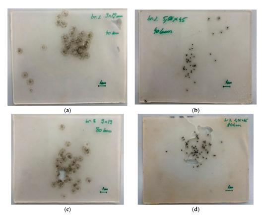
**Figure 6.** Ballistic tests with different calibers, (**a**,**c**) 9 mm and (**b**,**d**) 5.56 mm. The tests (**a**,**b**) were performed with 40 shots and (**c**,**d**) with 80 shots (the scale in the lower right corner shows 1 cm.
