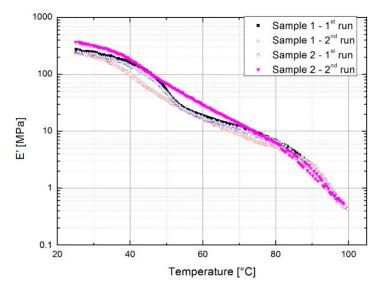
**Figure 2.** Storage modulus of the neat polymer. In the first run, samples were heated either to 89 °C (Sample 1) or 98 °C (Sample 2).
