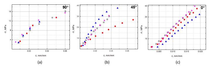
**Figure 3.** Results of flexural bending tests on composite reinforced with a double layer of fibers in three directions: (**a**) in the 90°, (**b**) in the 45° direction and (**c**) in the 0° direction, with respect to UD fibers orientation (four samples tested for each direction, each data set is presented with a different symbol).
