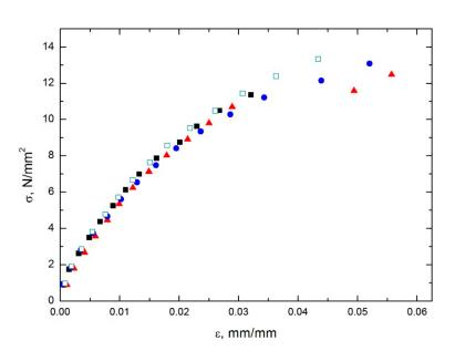
Figure 5. Results of tensile tests on the neat polymer.
