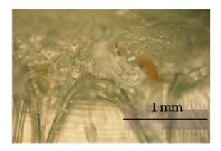
**Figure 7.** Scar after the ballistic test—transparency of the material is lost and there are visible copper particles.
