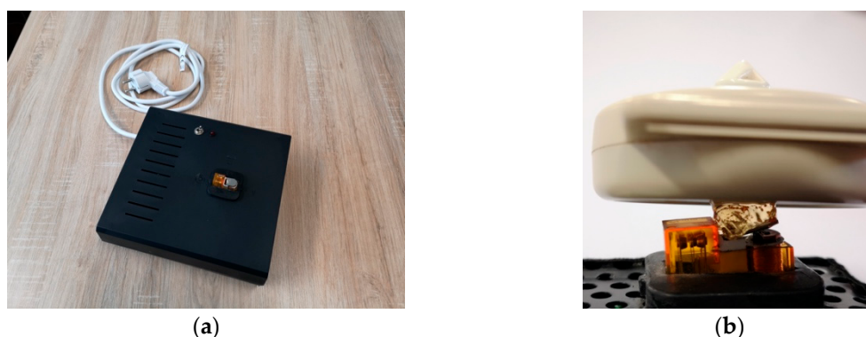
Figure 11. Final prototype of the fetal heart rate simulator device: (a) fetal heart rate simulator device, and (b) relay and US probe during simulation tests.
