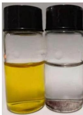
Figure S9. The photograph of polyiodide solutions without fiber (left) and with GC-PAN/I (1:0.25) (right) after standing for 24 h.
