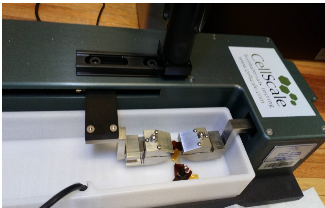
Fig. 1. Tensile mechanical testing of zirconia/Nafion ® nanocomposite membrane (a) Clamp; (b) specimen - pure Nafion ® membrane and Nafion ® /ZrO 2 nanocomposite membrane.
