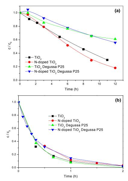
**Figure 6.** Disappearance of clopyralid (1.0 mmol/dm<sup>3</sup>) under visible (a) and UV (b) light irradiation (1.0 mg/cm<sup>3</sup> of catalyst).
