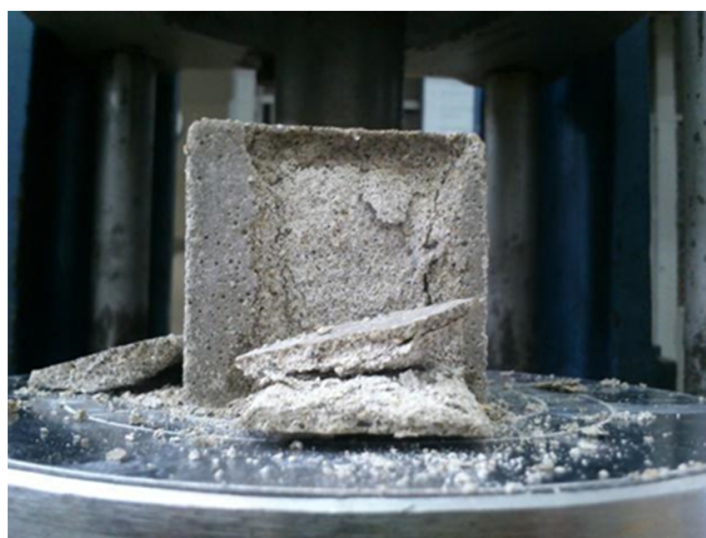
Figure 4. Illustration of the compressive strength test.
