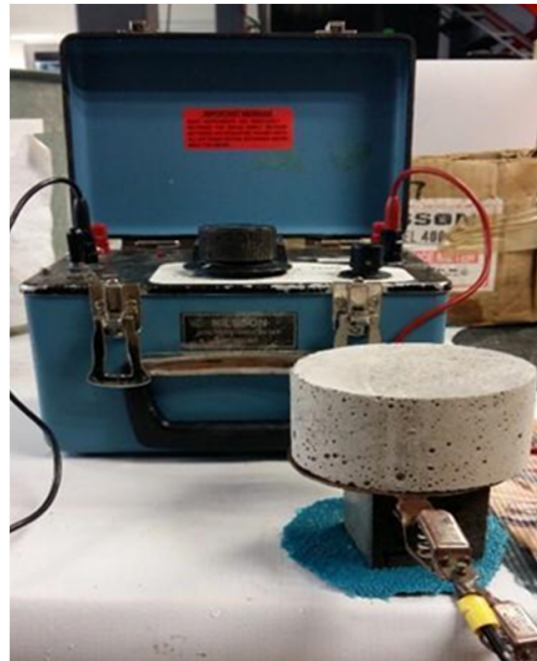
Figure 5. Illustration of the electrical resistivity test and equipment.
