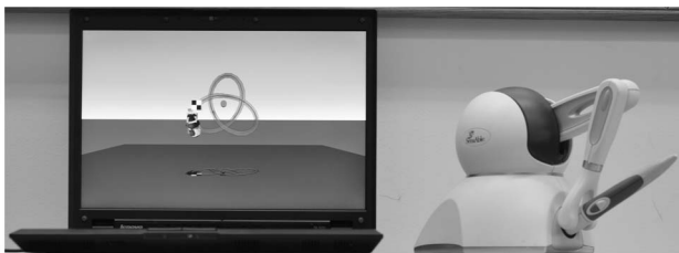
Figure 2. The PHANTOM Omni with the display. The display shows the path used in baseline and posttest trials. doi:10.1371/journal.pone.0092464.g002
