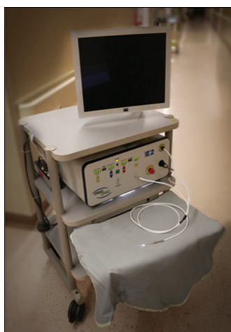
Figure 2: An endoscopy and laser unit used at the hospital for sick children, Toronto, housing a Xenon light source, diode laser, video camera and display screen, with the endoscope probe attached
