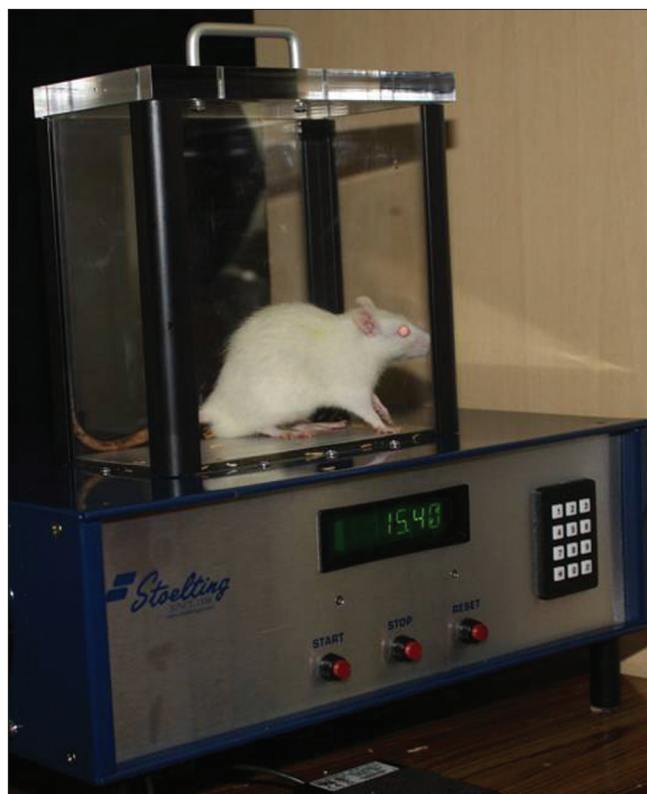
Figure 1: The hot-plate apparatus from Stoelting, USA used for testing pain response in the form of licking of hind paw or jumping. The cut-off time was 45 seconds
