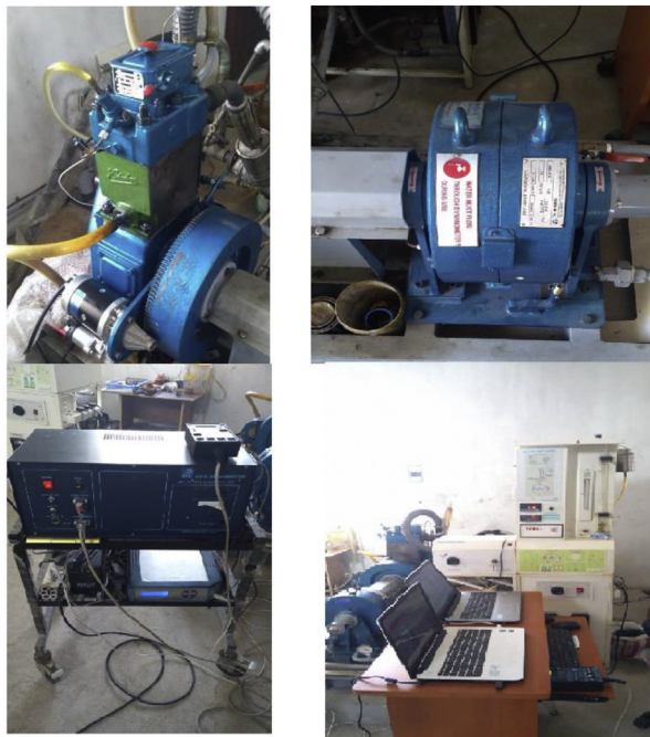
Fig. 2. Photograph of experimental test rig, dynamometer, smoke meter with gas analyser and computerized test rig.
