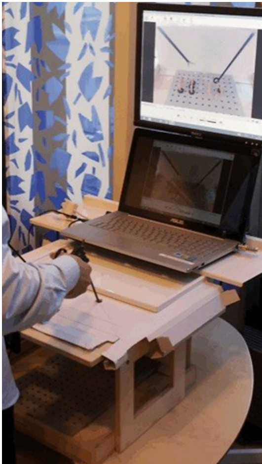
Fig. 1 The BlackBox; a box consisting of wood-material, with three holes in the roof, one for a camera and two for the laparoscopic instruments
