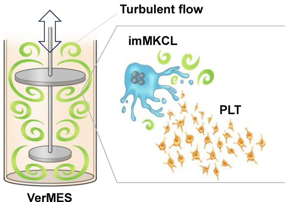
**Fig. 2.** Turbulence-based bioreactor, VerMES. Vertical reciprocal motion by the mixing impellers with optimized speed produces turbulent flow with optimal shear stress, which improves the yield and quality of the PLTs.
