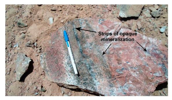
**Figure 5.** A hand specimen showing parallel bands of iron oxides with high radioactivity minerals (phase-II), associated with quartz veinlets.
