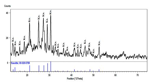
Figure 12. XRD pattern of Kasolite, El Urf mineralized pegmatite (phase-II).
