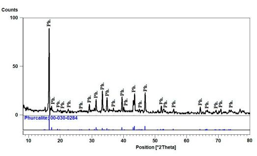
Figure 10. XRD pattern of Phurcalite, El Urf mineralized pegmatite (phase-II).
