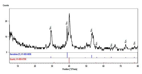
Figure 13. XRD pattern of xenotime, El-Urf mineralized pegmatite parts (phase-I).
