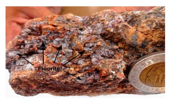
**Figure 6.** A hand specimen showing iron oxides associated with megacrystals of colorless and purple fluorite with high radioactivity minerals (phase-II).
