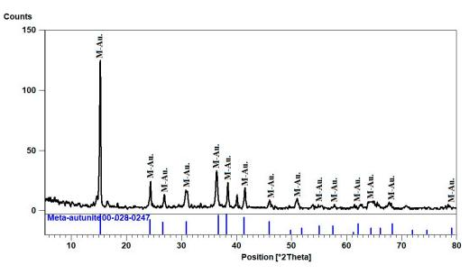
Figure 11. XRD pattern of Meta-autunite, El Urf mineralized pegmatite (phase-II).
