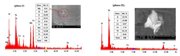
Figure 8. EDX-analysis of thorite, El-Urf mineralized pegmatite (phase-I), and (phase-II).
