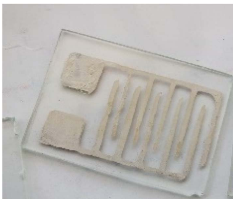
Fig. 3 Interdigitated silver-based electrode on glass substrate.
