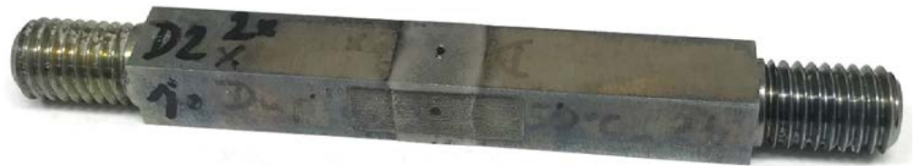
Figure 3. Example of the sample used for the physical simulation of the welding process (the figure shows a sample after the application of the temperature cycle of 1386 °C).
