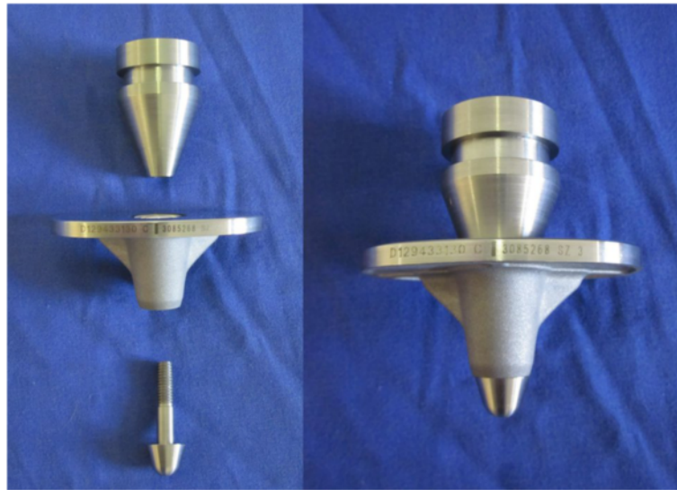
Figure 2 Modification for testing of MB trays: disassembled (left) and assembled (right).
