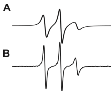
Figure 1. Representative electron paramagnetic resonance (EPR) spectrum of an intact spin-labeled protein (A) and that of the cleaved pieces with spin labels attached (B). The smaller the cleaved protein piece, the sharper the continuous wave (CW) EPR spectrum.
