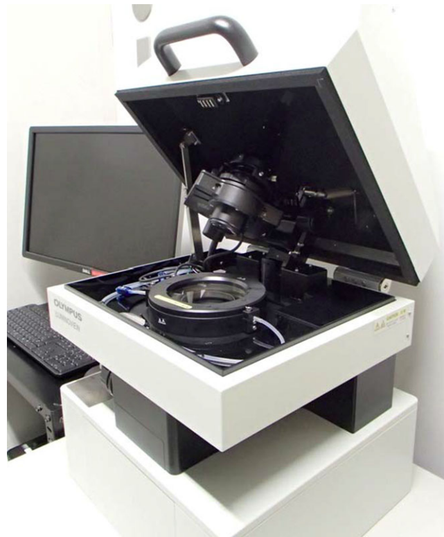
Fig. 1. Bioluminescence microscope, LV200. The stage-top incubator with temperature and CO 2 gas controller was added on the sample stage. The observation area was covered with a dark box.
