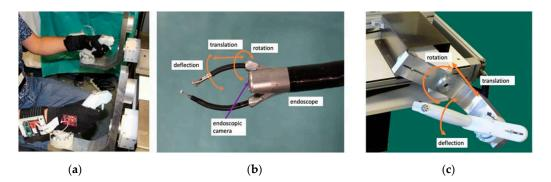
**Figure 2.** Expert wearing the sensor gloves while manipulating the robotic master/slave system (**a**). Master-slave control chart of the master/slave system (**b**). Direction and type of tool-tip and control movements (**c**).
